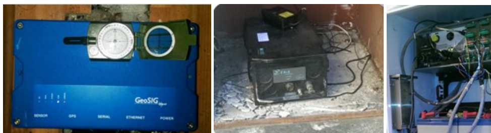
Fig. 2. Digital functional stations (GeoSIG GMS-18 station - left, ETNA - centre and Granite Kinematics Station - right)
